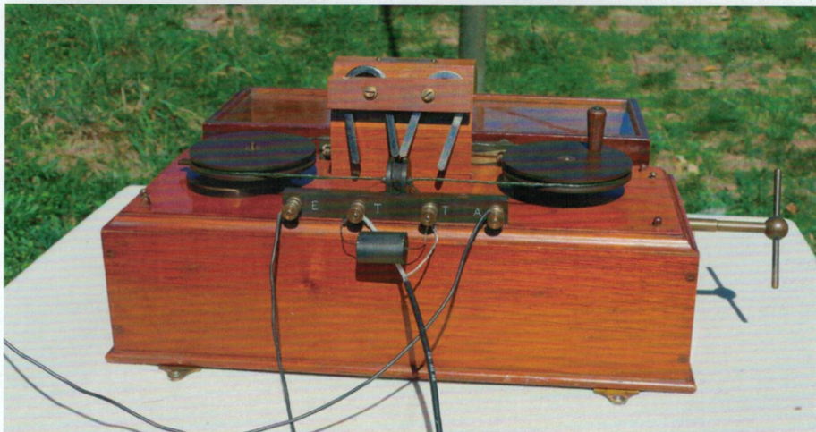
Photo N° 9 the magnetic detector in operation
