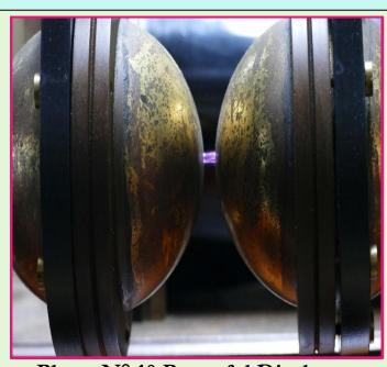
Photo N° 10 Powerful Discharge between the Central Balls
