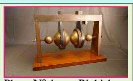
Photo N° 4 type Righi 4 balls oscillator
