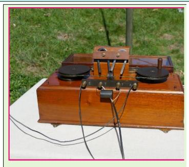
Photo N° 9 the magnetic detector in operation
