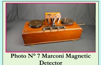
The most suitable receiver for this experience was considered the Marconi Magnetic detector (Photo N° 7) produced by Marconi Wireless Telegraph Co Ltd since 1902.
