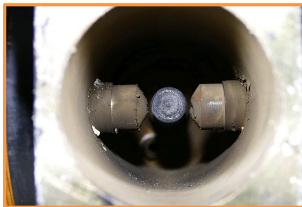
The arc chamber: in the foreground the polar masses and in the center the carbon cathode
