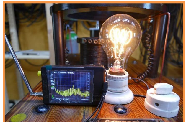
The system starts to oscillate at 1.200 kHz, the I1 bulb with dummy load function lights up vigorously
