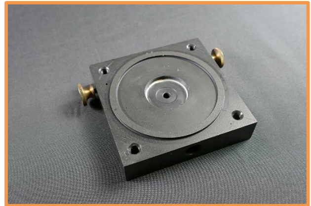
Platinum membrane seat with application of sealing mastic
