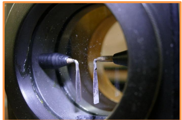
B and C plates in TP 316 stainless steel
