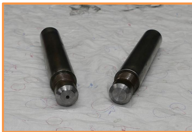
The polar masses after the turning operation
