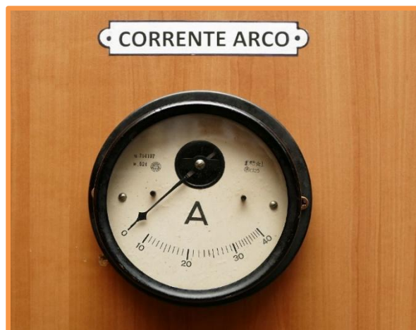
The ammeter used to measure the arc current
