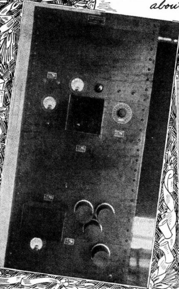
Early Farnsworth cathode-ray television transmitting and receiving system about 1931.
